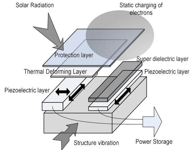
**Fig1. The new integrated energy harvesting system**
