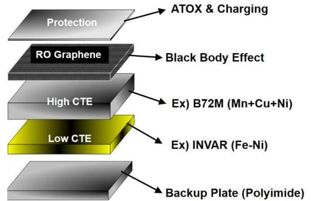
Fig. 3 Structure of the bimetal element
