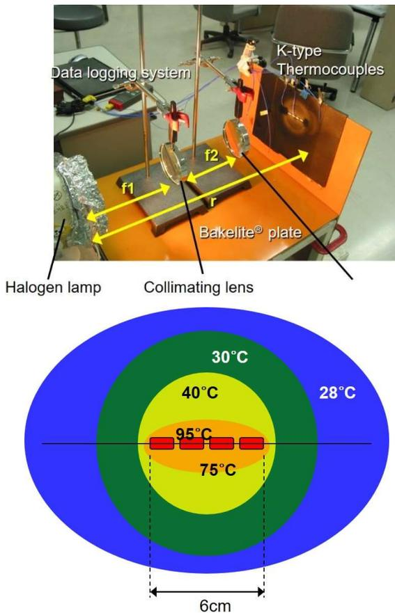
**Fig. 4 Simple Simulator of Solar Radiation and Test result of heating effect using two convex lenses.**
