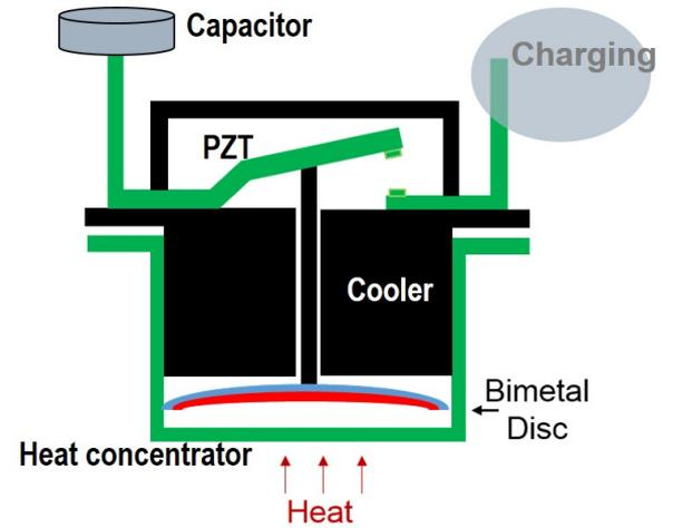
Fig.2 Bimetal-PZT energy harvesting system
