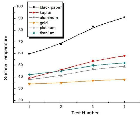
**Fig. 5 Common material used in space mission tested for heating temperature**
