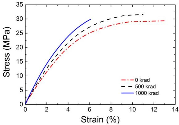
**Fig. 7.** Typical 3-point bending stress-strain curves of printed samples with post curing for 60 min at 275°C in N<sub>2</sub> atmosphere before and after exposure to  $\gamma$  radiation.
