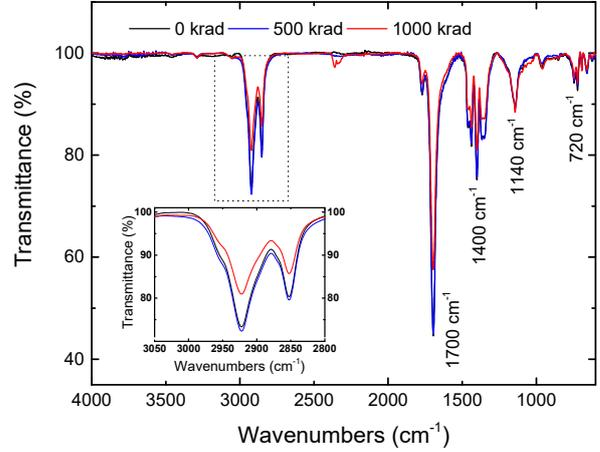
**Fig. 8.** FTIR measurements of printed samples (post cured for 60 min at 275°C in N<sub>2</sub> atmosphere) before and after exposure to  $\gamma$  radiation: unexposed (black); after 500 krad (blue) and after 1000 krad (red) radiation dose.
