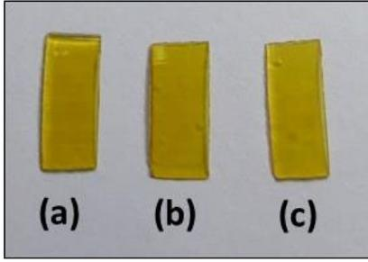
**Fig. 6.** Images of the printed samples with post curing for 60 min at 275°C in N<sub>2</sub> atmosphere before and after exposure to  $\gamma$  radiation: (a) unexposed, (b) 500 krad, (c) 1000 krad.
