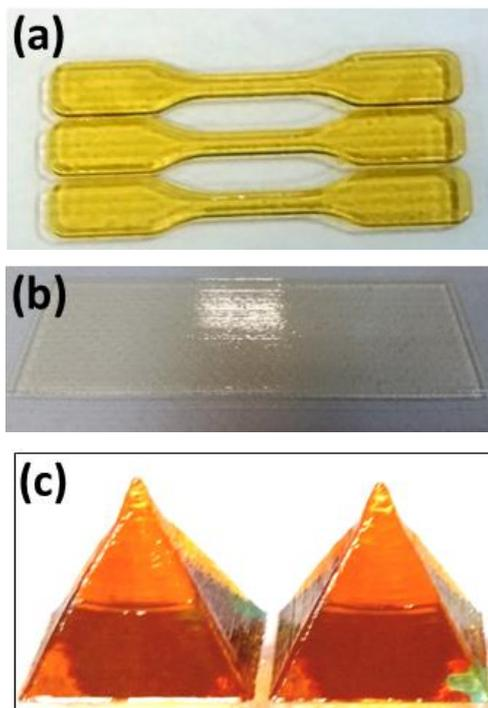
**Fig. 4.** 2D-like and 3D printed PI samples: (a) 1.5 mm thick – "dog bone"; (b) 300 μm – thick film; (c) 1 cm – height pyramid
