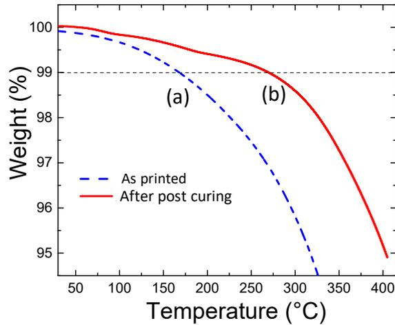
**Fig. 5.** TGA measurements (5°C/min in N<sub>2</sub> atmosphere) of printed PI: (a) without post curing; (b) after post curing for 60 min at 275°C.
