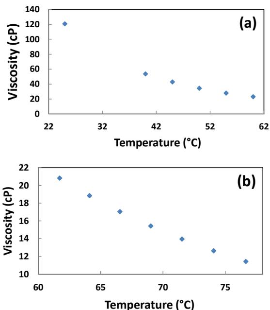
**Fig. 2.** Viscosity of PI-based ink as function of temperature: (a) measured values, (b) extrapolated to relevant working range.
