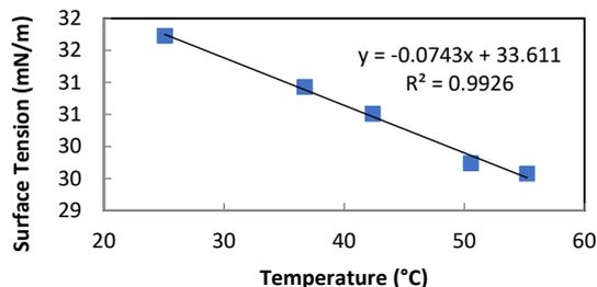
**Fig. 3.** Static surface tension of PI-based ink at different temperatures, as measured by a Force Tensiometer.
