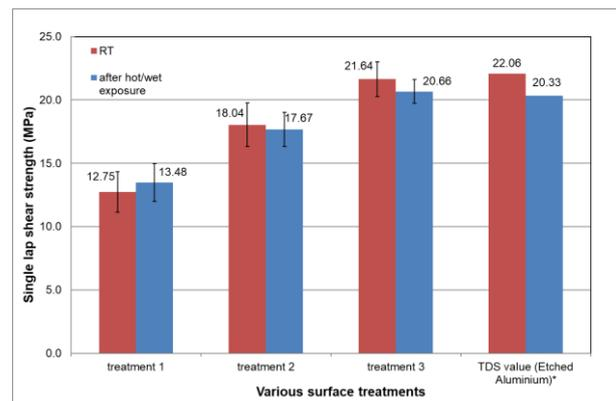
Figure 1: Single lap shear strength for post-cured ScotchWeld 2216 on FeNi36 alloy (INVAR®) before (red bars) and after exposure to "hot-wet" conditions (blue bars) as a function of surface treatment<sup>1</sup>
