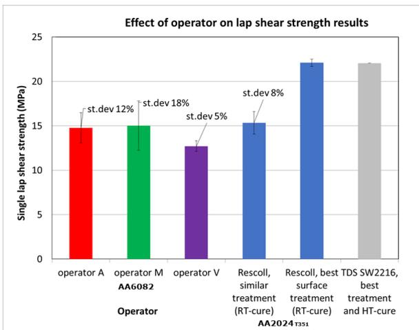
Figure 4: The operator's influence on the adhesive bonding reflected in the adhesive shear strength (first three from the left), compared with reference values from other tests (blue
