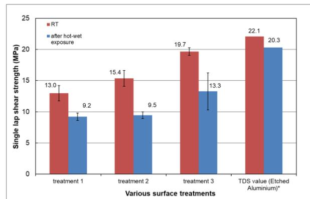
Figure 3: Single lap shear strength of RT-cured ScotchWeld 2216 on aluminium substrate before (red) and after “hot-wet” exposure (blue) as a function of surface treatment \*.
