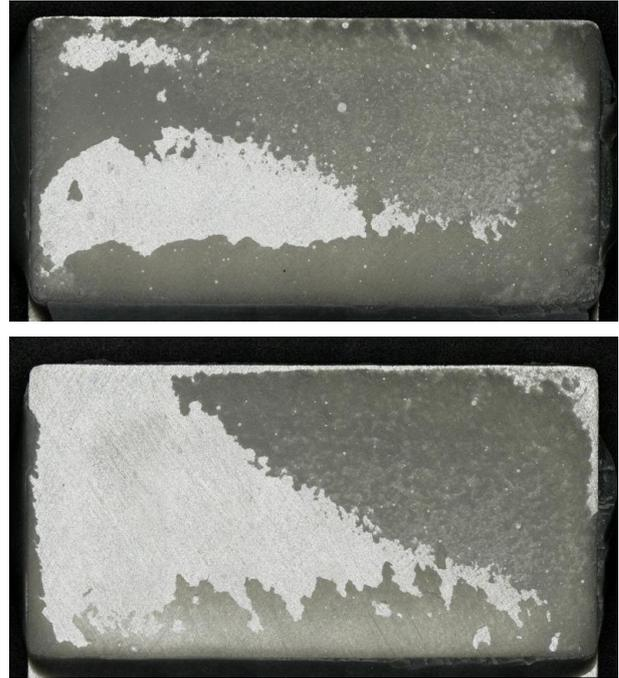
Figure 5: The analysis of fracture surfaces from the samples with the highest (top) and the lowest (bottom) shear strength.
