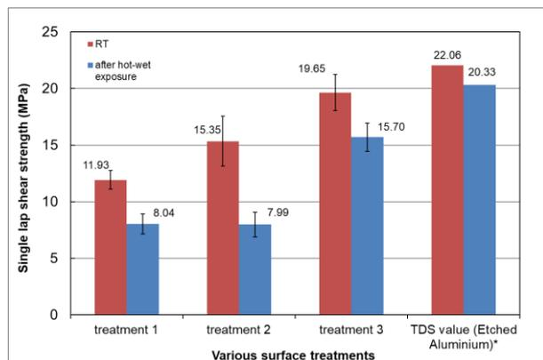
Figure 2: Single lap shear strength of RT-cured ScotchWeld 2216 on FeNi36 alloy (INVAR®) before (red bars) and after “hot-wet” exposure (blue bars) as a function of surface treatment.
