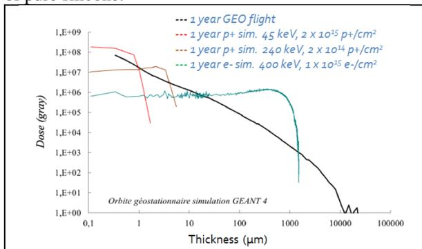
**Fig. 3.** Particles simulation depth penetration for a silicone ( $d = 1.2$ ) – calculation [8]
