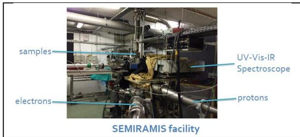
**Fig. 2.** Picture of SEMIRAMIS facility at ONERA
