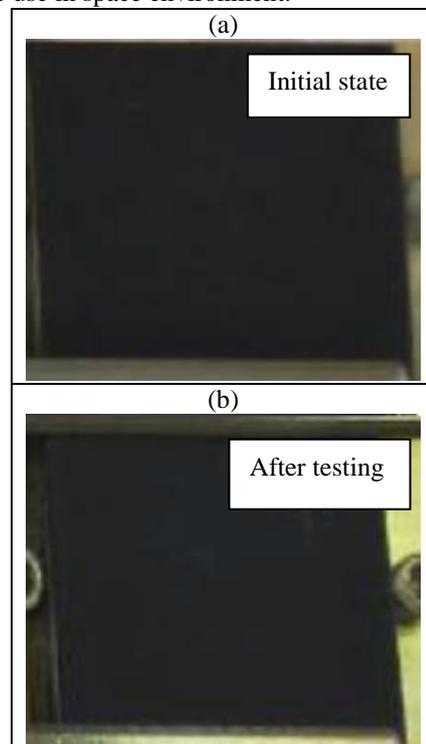
**Fig. 5.** Pictures of MAP<sup>®</sup> HT1607 sample (a) before and (b) after GEO irradiation
