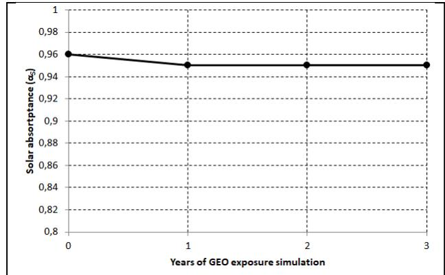
**Fig. 4.** Evolution of the solar absorptance versus duration of exposure to the GEO simulated environment
