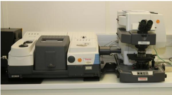
**Fig. 1.** Picture of the Thermo Fischer Nicolet 6700 and Continuum Imaging System
