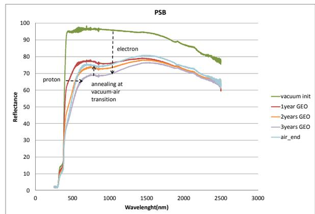
**Fig. 4** – Reflectance curves at 1, 2 and 3-year GEO doses and after venting (air\_end) for PSB (2016)
