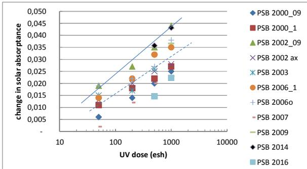
**Fig. 6** - Change in solar absorptance of PSB with UV dose. Straight/dashed lines are respectively upper bound limit and mean degradation.
