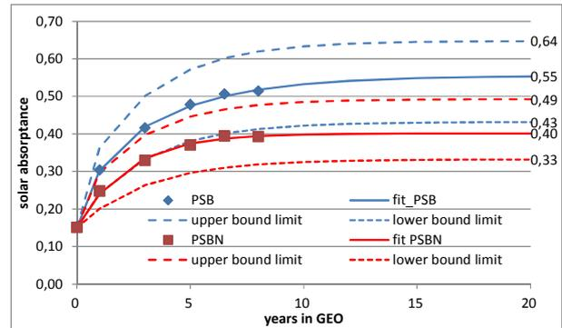
**Fig. 10 – Extrapolated solar absorptance of SG121FD (top) and PSB/PSBN (bottom) accounting for variability of data.**
