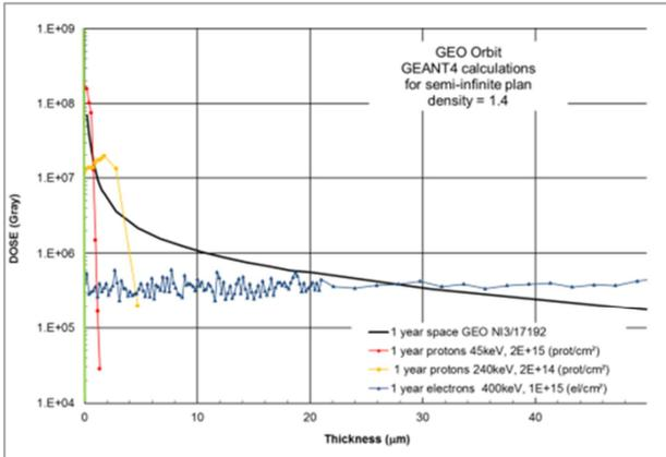
**Fig. 1** – GEO dose profile at SEMIRAMIS combining electrons (bulk dose), protons and UV exposure (surface dose). Provided fluence here are calculated for a 1-year mission.
