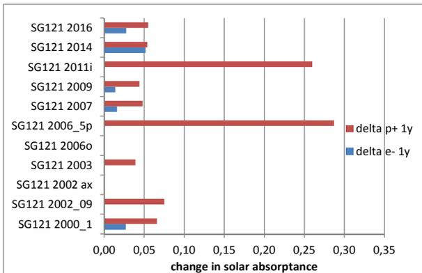
**Fig. 7** – Change in solar absorptance after 1-year electron (e-) and proton (p+) doses for SG121FD.
