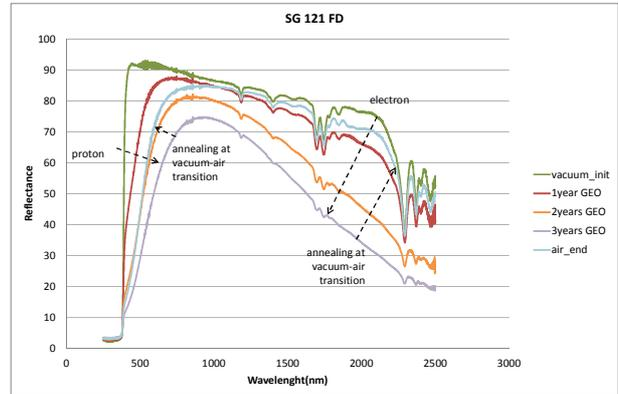
**Fig. 3** - Reflectance curves at 1, 2 and 3-year GEO doses and after venting (air\_end) for SG121FD (2016)
