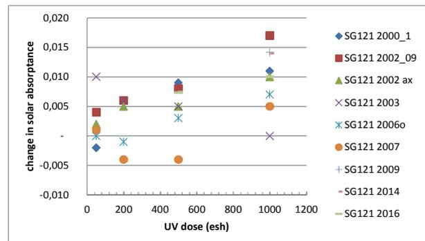
**Fig. 5** - Change in solar absorptance of SG121FD with UV dose.
