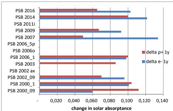
**Fig. 8** – Change in solar absorptance after 1-year electron (e-) and proton (p+) doses for PSB.
