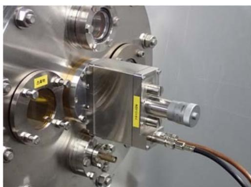
Figure 2 Rectangular shape pulsed supersonic valve developed in this study (upper panel) and single-PSV configuration (lower panel)
