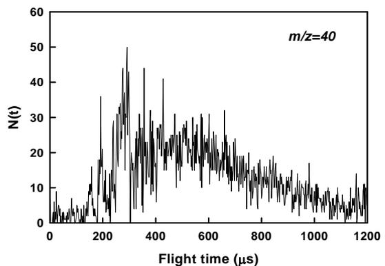
Figure 7 Time-of-flight spectra of hyperthermal thermal AO and Ar beams detected by QMS in dual-PSV configuration; upper panel:  $m/z=16$  and lower panel:  $m/z=40$
