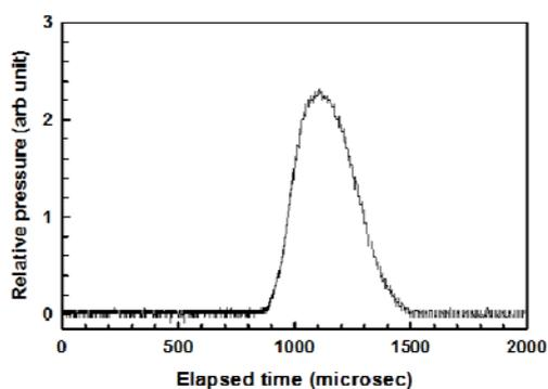
Figure 3 Pressure profile of new PSV measured in atmospheric condition
