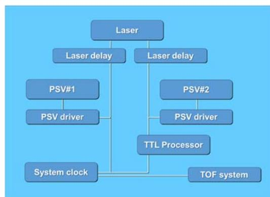
Figure 5 Block diagram of dual-PSV configuration
