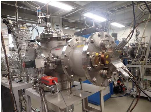
Figure 1 One-Nozzle two-beam laser detonation beam facility used in this study
