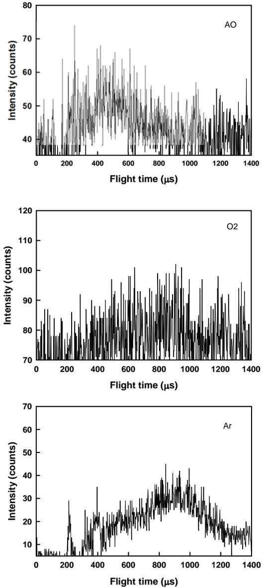
Figure 2 Time-of-flight spectra of AO, O<sub>2</sub> and Ar beams (From top to bottom). Average translational energies are 2.9, 4.0 and 4.0 eV, respectively.
