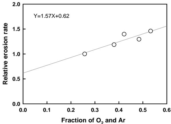
Figure 3 Relationship between Ar+O<sub>2</sub> fraction in the beam and the relative erosion rate of polyimide.
