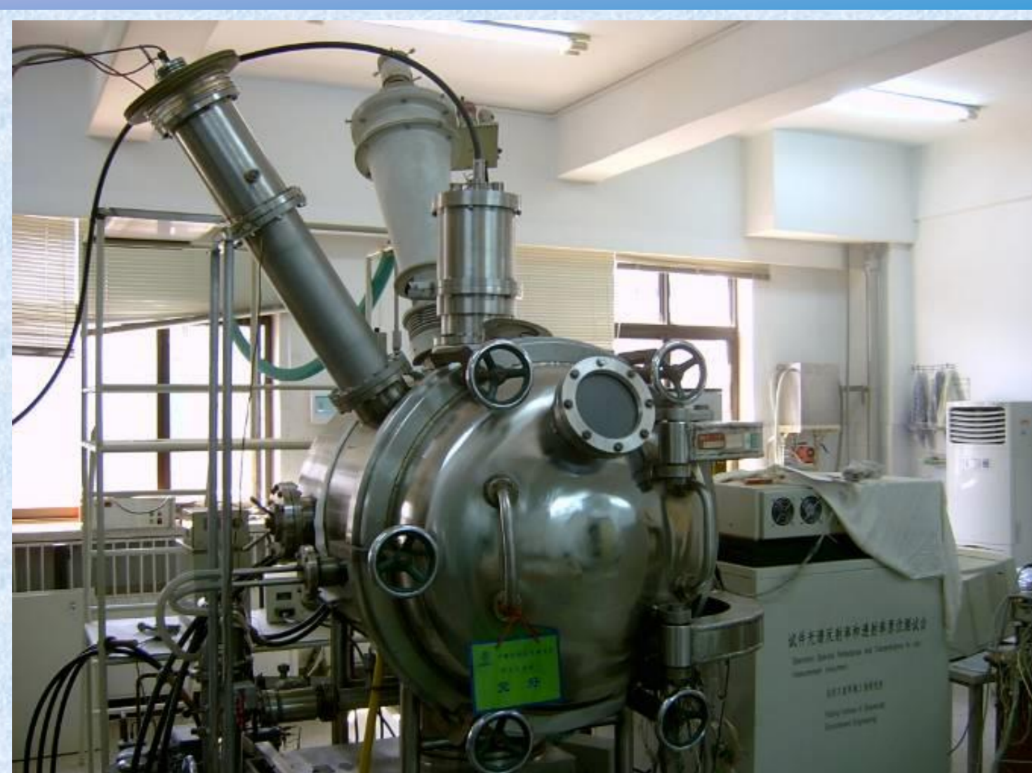
Low-energy combined environment test facility at Beijing Institute of Spacecraft Environment Engineering (BISSE)
