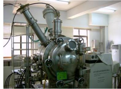
Fig.1. Low-energy combined environmental test facility
