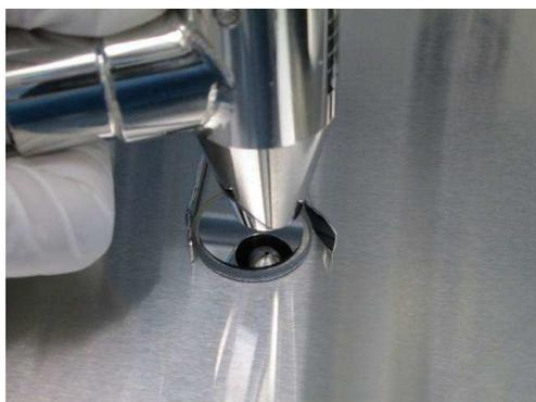
**Fig.4.** Example of decontamination via atmospheric ultrasonics
