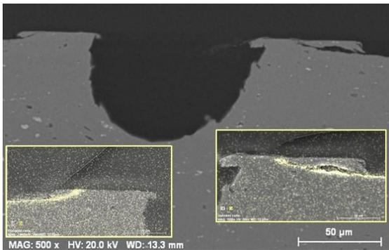
**Fig. 6 :** SEM image with EDS mappings of a metallographic section of crater (B)
