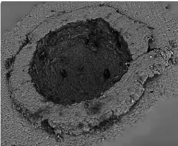
**Fig. 2** : 3D representation of crater (A) after reconstruction. Obtained by SEM images in BSE mode
