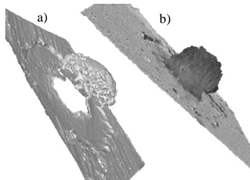
**Fig. 4** : Backside 3D representation of crater (B) after reconstruction by confocal optical profiler (a) and 3D SEM (b)
