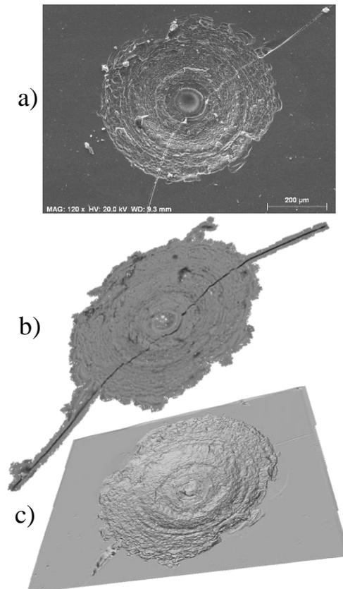
**Fig. 7 :** Characterization of a crater into a coverglass: SEM image a) 3D SEM reconstruction b) and confocal profiler representation
