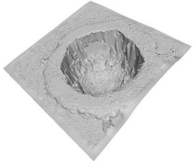
**Fig. 3** : 3D representation of crater (A) obtained by confocal optical profiler
