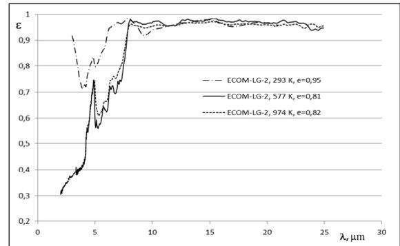
**Fig.7.** Spectral emittance of ECOM-LG-2 (white coating) measured at three temperatures.
