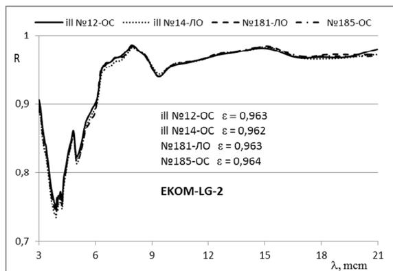
**Fig. 11.** Reflectance spectra of ECOM-LG-2 samples in the wavelength range from 3 to 20 μm (before (witness) and after full-scale exposure)
