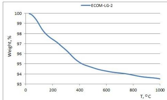
**Fig.4.** Thermogravimetric analysis of ECOM-LG-2
