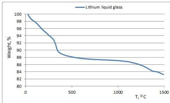
**Fig.6.** Thermogravimetric analysis of lithium liquid glass-based binder
