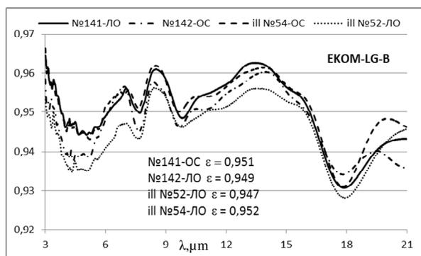
**Fig.12.** Reflection spectra of ECOM-LG-B samples in the wavelength range from 3 to 20 μm (before (witness) and after full-scale exposure)
