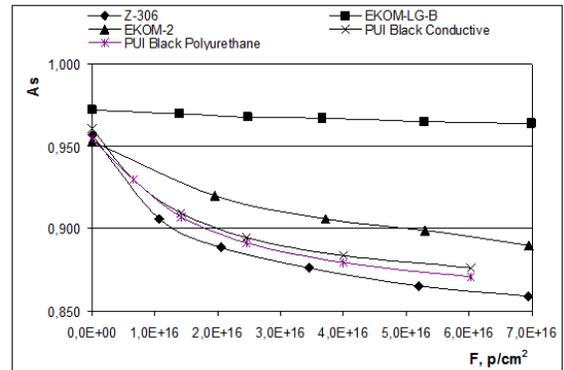
**Fig.3.** Dependence of solar absorptance of ECOM-LG-B on  $F_p$  at simultaneous irradiation by protons + electrons + solar UV.
