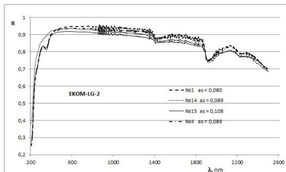
**Fig. 14.** Reflectance spectra of ECOM-LG-2 samples (before and after O-plasma experiments)
