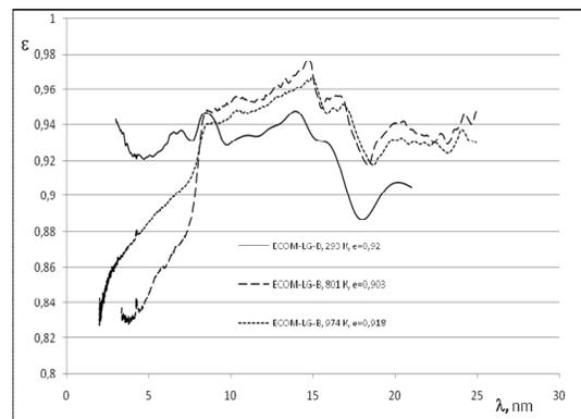
**Fig .8.** Spectral emittance of ECOM-LG-B (black coating) measured at three temperatures.
