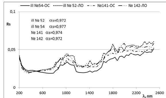
**Fig.10.** Total reflectance spectra of ECOM-LG-B samples in the wavelength range from 0.2 to 2.5 µm (before (witness) and after flight experiments)
