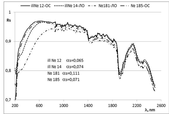
**Fig.9.** Total reflectance spectra of ECOM-LG-2 samples in the wavelength range from 0.2 to 2.5 µm (before (witness) and after flight experiments)
