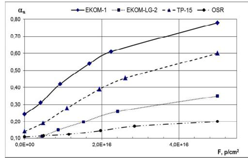
**Fig. 2.** Dependence of solar absorptance of ECOM-LG-2 on  $F_p$  at simultaneous irradiation by protons + electrons + solar UV.
