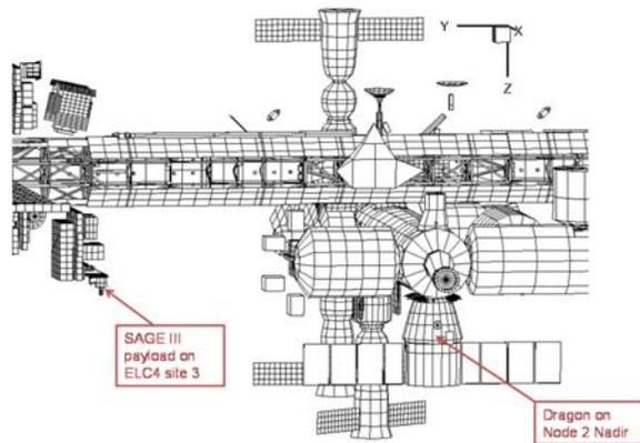
**Figure 8.** SAGE III and the Dragon cargo vehicle on ISS
