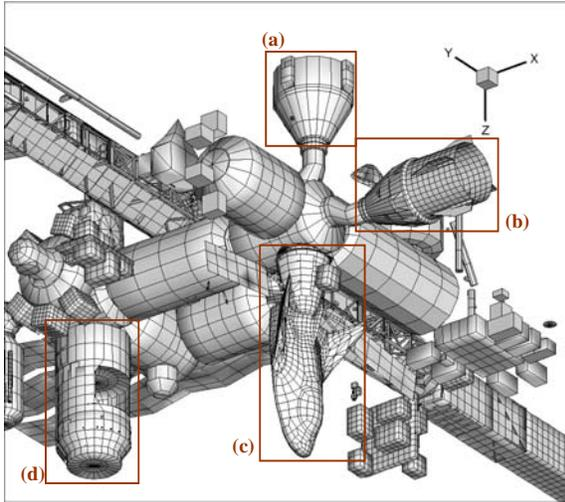
**Figure 2.** U.S. Segment docking and berthing ports
