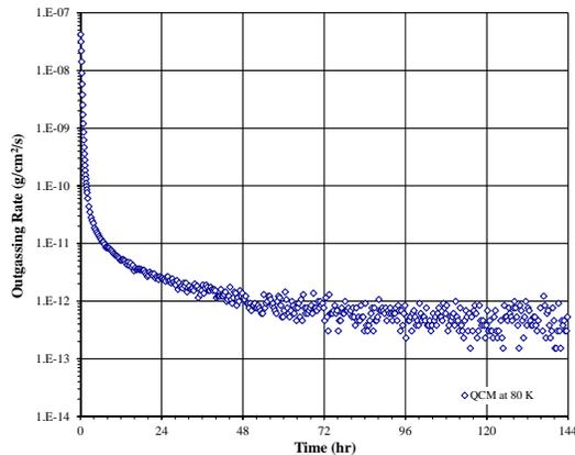
**Figure 5.** Example ASTM E1559 outgassing rate data.
