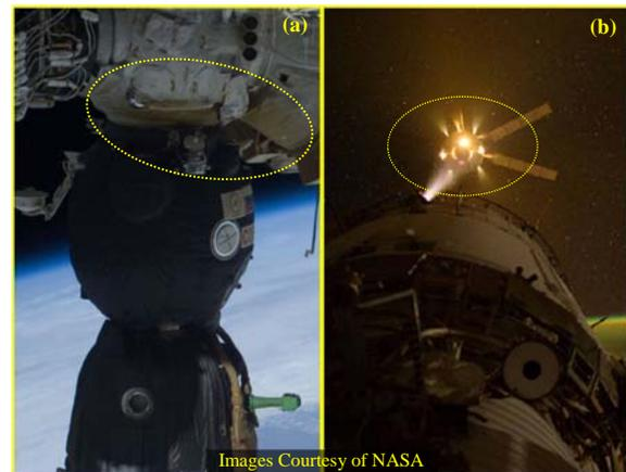
**Figure 1.** Visiting vehicle contamination sources
