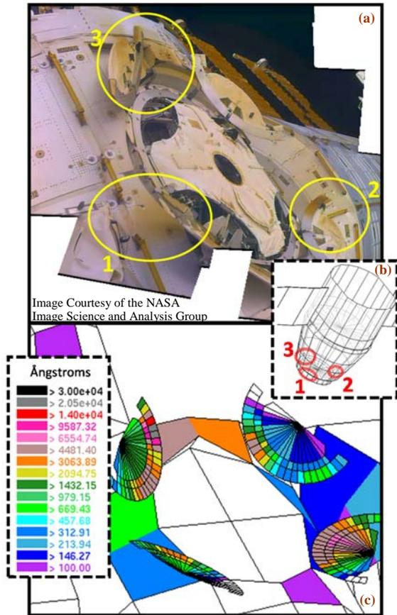
**Figure 7.** Discoloration of the Node 2 nadir CBM due to visiting vehicle materials outgassing
