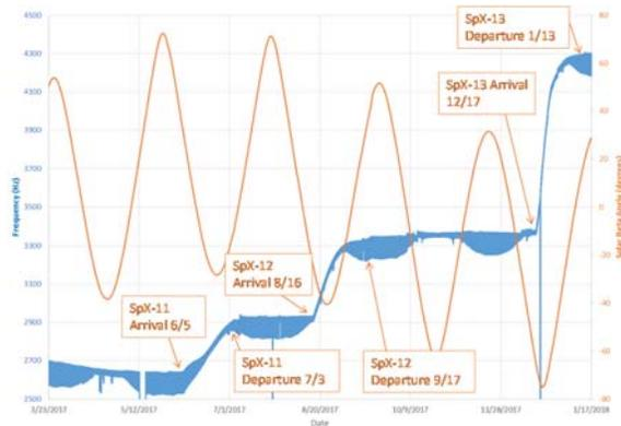
**Figure 9.** Example SAGE III QCM Frequency Data
