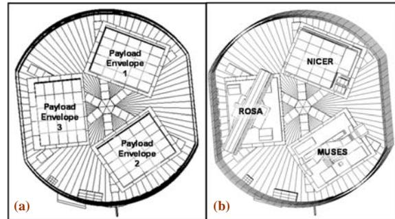
**Figure 6.** Example visiting vehicle cargo volume models used for materials outgassing analyses
