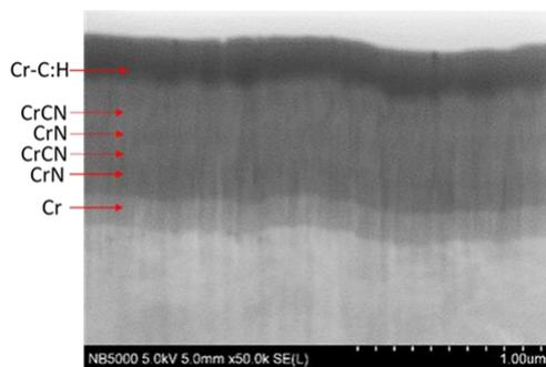
**Fig. 2.** Cross section of Cr/CrN+CrCN/Cr-C:H (DLC1) coating produced on CuBe2 tape.
