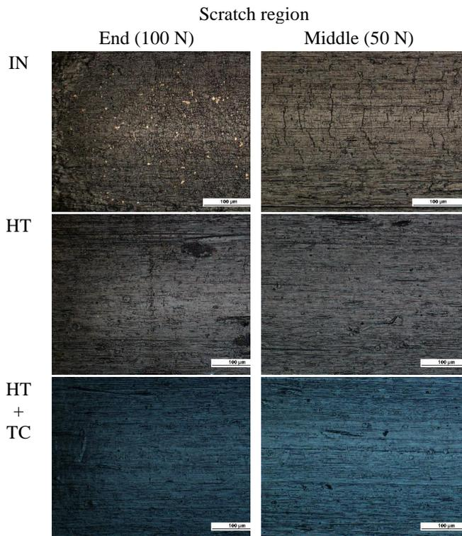
**Fig. 12.** The appearance of scratches performed on DLC3 coating produced on CuBe2 substrate after different treatments.
