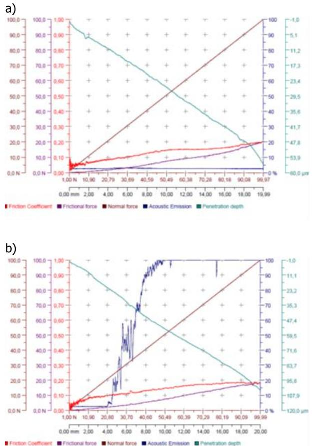
**Fig. 11.** Graphs obtained for scratch test of DLC3 coating before (a) and after (b) heat treatment (red – friction coefficient, blue – acoustic emission signal, green – penetration depth).
