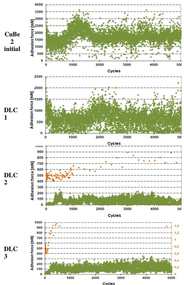
**Fig.7.** Adhesion force and friction coefficient evaluation through 5,000 cycles.
