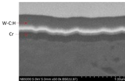
**Fig. 3.** Cross section of Cr / W-C:H (DLC2) coating produced on the CuBe2 tape.
