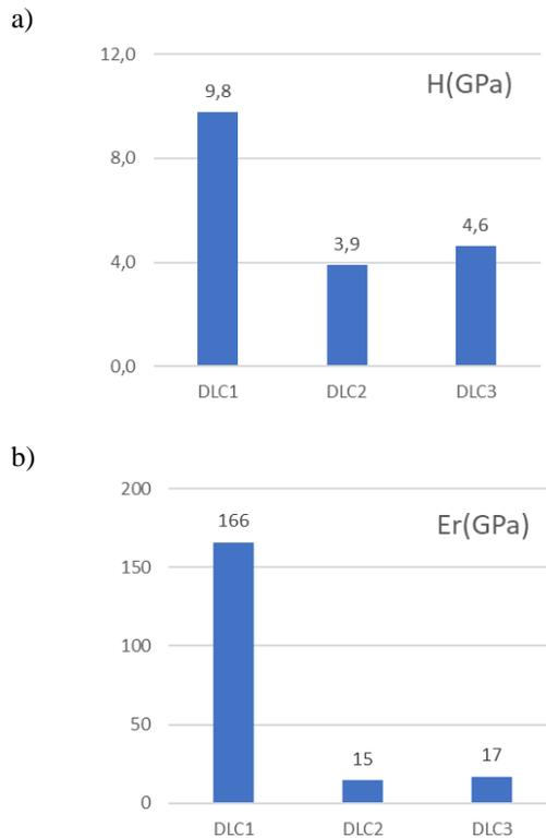
**Fig. 10.** Microhardness (a) and Young's modulus (b) equal values for DLC coatings produced on CuBe2 substrate.
