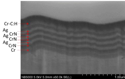
**Fig. 4.** Cross section of Cr/CrN+Ag/Cr-C:H (DLC3) coating produced on CuBe2 tape.
