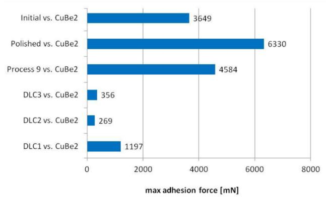
**Fig. 9.** Maximum adhesion force measured during 5,000 cycles.
