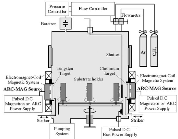
**Fig. 1.** Deposition chamber equipped with two planar ARC-MAG sources and substrate holder with planetary rotation.
