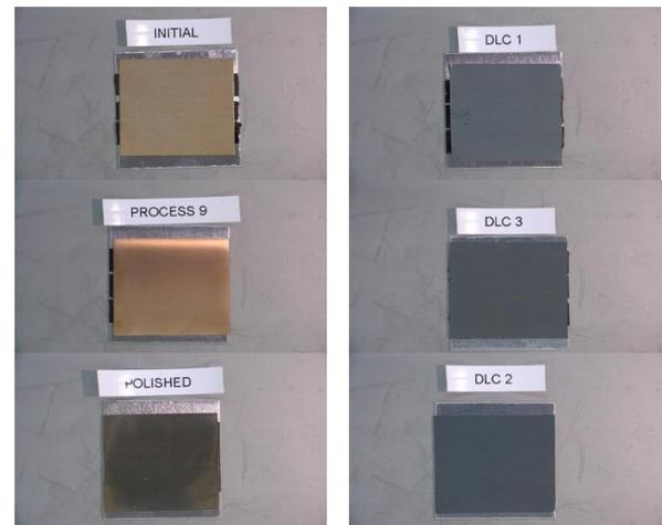
**Fig. 5.** DLC coated and mechanically modified CuBe2 samples used for thermo-optical measurements.
