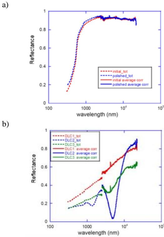
**Fig. 6.** Total reflectance spectra in solar wavelength range 300–2,500 nm and in infrared wavelength range 2.5–20  $\mu\text{m}$  for DLC coatings and CuBe2 tape.
