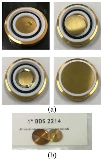
**Figure 3** Sample holders available for BDS (a) and RF (b) testing at ESTEC.
