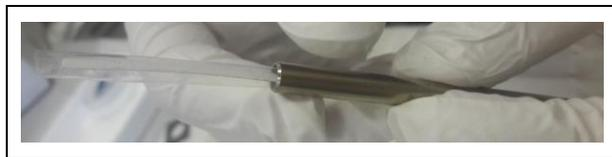
**Fig. 1.** Material sample inserted into PTFE liner and stainless steel ATD tube
