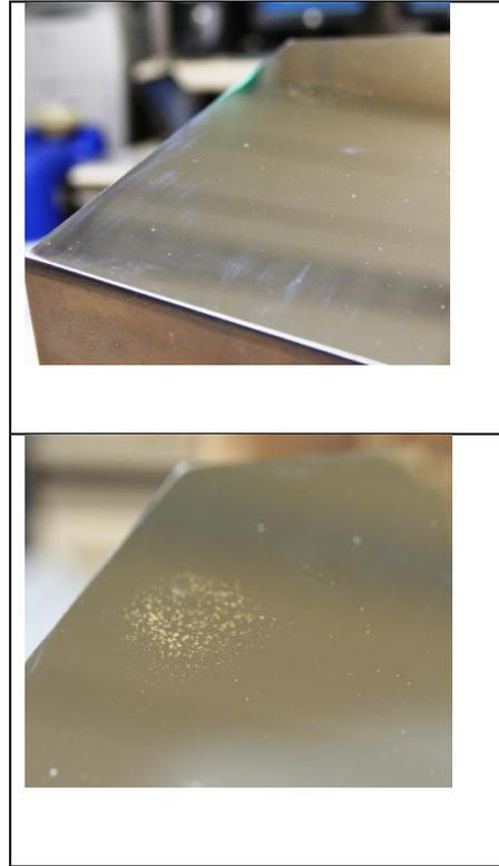
Figure 17 Defects observed on a mirror surface showing the influence of lighting conditions and angle of illumination. In the upper image, cleaning residue and streaks can be seen on the surface. In the lower image, the mirror was tilted slightly to reveal an area of delamination (ESA)
