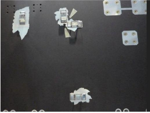
Figure 9 Delamination of black paint on a structural panel, at sharp edges next to cable clamps (ESA/Airbus)
