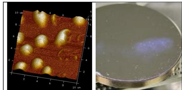
Figure 4 Defects in the SiO<sub>2</sub> coating on a Beryllium mirror after high energy proton radiation test (ESA)
