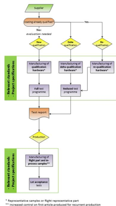
Figure 15 General test logic for evaluation and qualification of coatings (from ECSS-Q-ST-70-17C)
