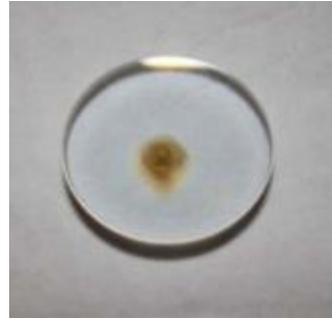
Figure 11 Typical damage on an AR coating sample due to laser induced contamination (ESA/DLR)
