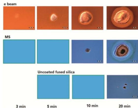
Figure 12 Optical micrographs showing the evolution of contamination induced damage on optical coatings manufactured with different coating technologies. The onset of damage is delayed on the Magnetron Sputtered (MS) coating, compared to the more porous e-beam coating (results from test with 500mJ/cm<sup>2</sup>, 1kHz laser) – ESA/DLR [7].
