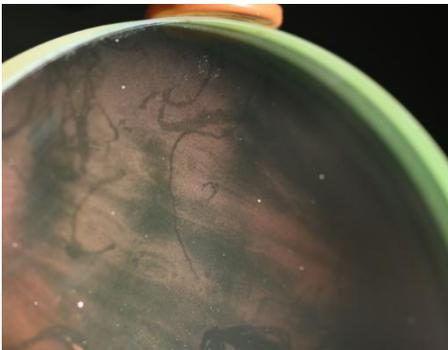
Figure 10 Stains on an optical filter due to substrate contamination prior to coating (ESA)
