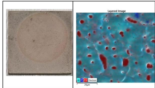
Figure 3 Evolution of copper within the coating after long term thermal ageing test (ESA)
