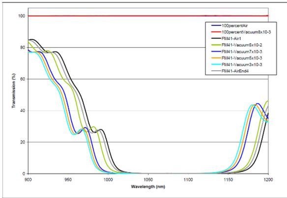
Figure 13 Example of air-vacuum wavelength shift observed in a high reflector coating at 1064 nm (ESA, reproduced from [2])
