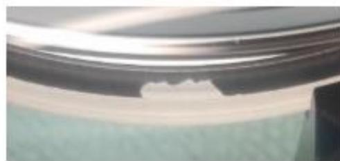
Figure 8 Delamination of black paint on the curved edge of an optical component (ESA/Airbus)
