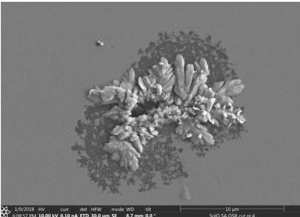
Figure 6 SEM micrograph showing localised delamination of the silver coating and growth of sulphur containing dendritic structure on an Optical Solar Reflector (OSR) after exposure to a standard cleanroom environment (ESA)
