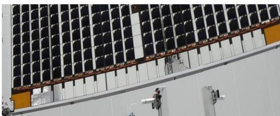
Figure 2 Edge shields with white thermal control coating on the Bepi Colombo Solar Array (ESA/Airbus)
