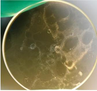
Figure 5 Degradation of an optical coating due to inadvertent condensation during a humidity test (ESA)
