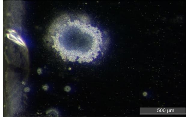
Figure 7 Localised corrosion of the silver coating on an Optical Solar Reflector (OSR) after a long duration humidity test (ESA)
