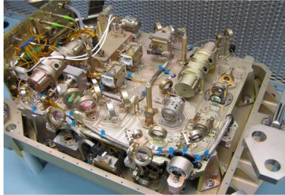
Figure 1 Thin film optical coatings are one of the most commonly used class of coatings for space application. The example shown here is the ALADIN laser instrument on the recently launched Aeolus satellite, which contains coatings on more than 80 optical surfaces ! (ESA/Leonardo Company)
