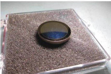
Figure 14 Degradation on an optical mirror due to incorrect storage of test sample in foam material (ESA)
