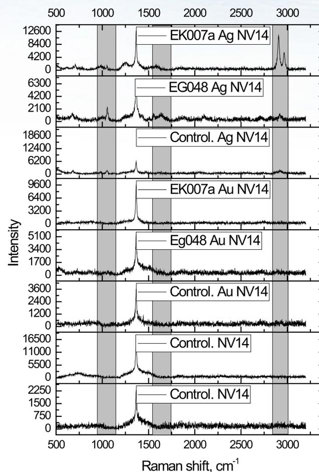
Figure 3. Results of investigation of SERS substrates based on ceramic coating NV14 in different laboratories
