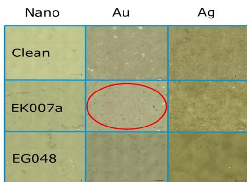
Figure 2. Optical pictures of of SERS substrates based on ceramic coating NV14 after 10 days of lab environment testing
