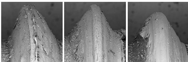
**Fig. 8.** Post 10 retightens (uncoated left, Molykote middle, CoBlast right)
