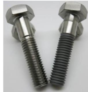
Fig. 1. Uncoated (left) and CoBlast coated (right) titanium bolts
