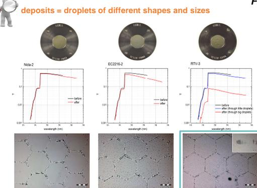
Fig 2. EUV transmittance of contaminated Al filters
