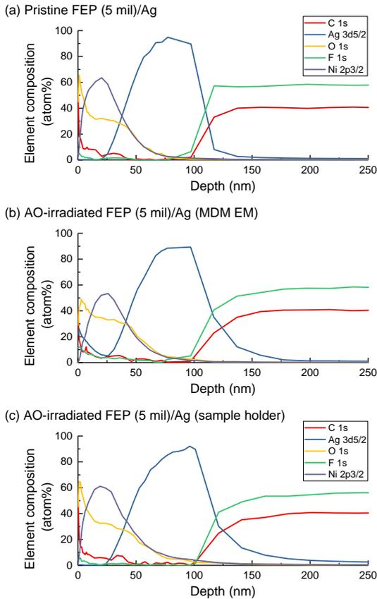
**Fig. 8** Depth profiles of the element compositions of the Ag (back) faces of the FEP (5 mil)/Ag (Ag face) samples obtained by the XPS: (a) pristine, (b) AO-irradiated on the MDM-EM, (c) AO-irradiated on the sample holder (depth: SiO<sub>2</sub> conversion; Etching: Ar beam (3 keV))
