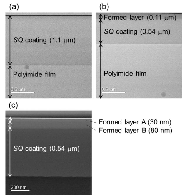
**Fig. 5** STEM images of the cross-section of the SQ coated polyimide films before (a) and after (b, c) exposure: (a), (b) BF (Bright Field) images, (c) HAADF (High Angle Annular Dark Field) image (acceleration voltage: 200 kV)
