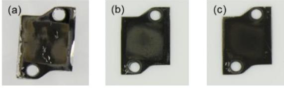
**Fig. 4** Back faces (Ag faces) of the silvered FEP films after exposure: (a) FEP (1 mil) film/Ag (installed position: 9), (b) FEP (5 mil) film/Ag (installed position: 11), (c) ITO/FEP (5 mil)/Ag (installed position: 13)
