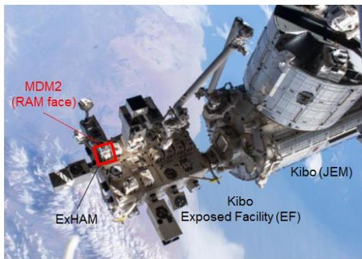
**Fig. 2** Positions of ExHAM and MDM2 sample holding part on Kibo Exposed Facility (EF)
