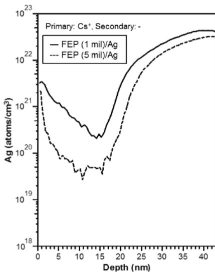
**Fig. 9** Depth profiles of the Ag density in Ni of the pristine FEP (1 mil)/Ag and the pristine FEP (5 mil)/Ag obtained by the SIMS (Ni standard sample was used for the quantification; primary ion: Cs<sup>+</sup> (2.0 kV))
