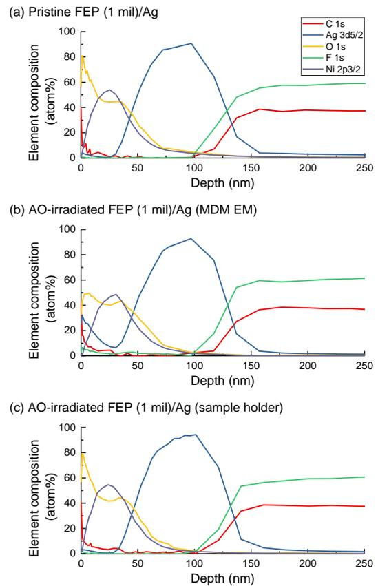
**Fig. 7** Depth profiles of the element compositions of the Ag (back) faces of the FEP (1 mil)/Ag (Ag face) samples obtained by the XPS: (a) pristine, (b) AO-irradiated on the MDM-EM, (c) AO-irradiated on the sample holder (depth: SiO<sub>2</sub> conversion; Etching: Ar beam (3 keV))
