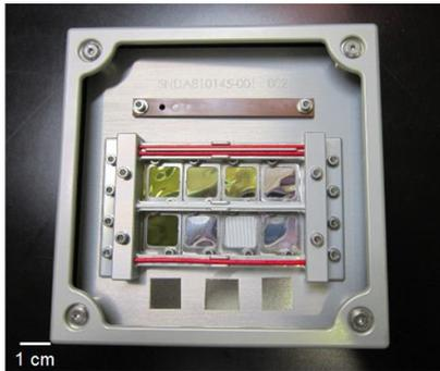
**Fig. 1** MDM2 sample holding part (exposed face; before space exposure)
