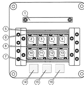
**Fig. 3** Positions of installed material samples on MDM2 sample holding part
