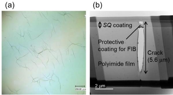
**Fig. 6** (a) Digital microscope image of the surface of the SQ coated polyimide films after exposure, (b) BF-STEM image of the cross-section of the SQ coated polyimide films (crack position) after exposure (acceleration voltage: 200 kV)
