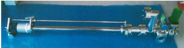
**Fig. 1.** Vacuum transfer vessel (VTV).
