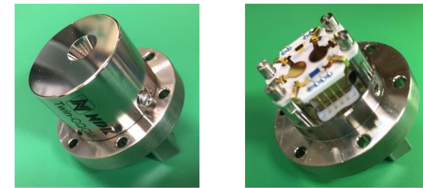
Fig. 2. Photos of the Twin-CQCM sensor unit (Left: unit with the cover; Right: unit without the cover)
