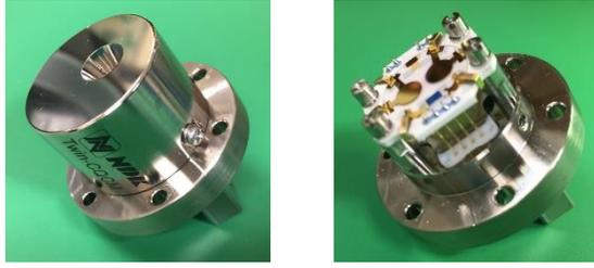
**Fig. 3.** Photos of the Twin-CQCM sensor unit (Left: unit with the cover; Right: unit without the cover)
