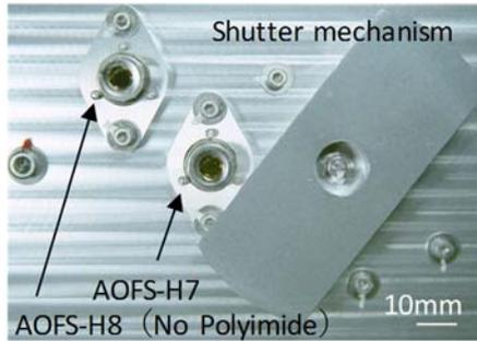
**Fig. 3.** AOFS sensors (AOFS-H7 and AOFS-H8) with shutter mechanism (installed on the X surface of SLATS)
