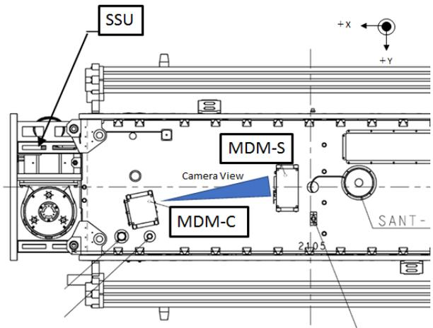
**Fig. 6.** Positions of MDM-S and MDM-C and the SSU (as viewed from the +Z side)
