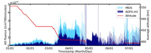
**Fig. 9.** Time dependence of AO fluence per orbit (every 90 min.) on the satellite -X plane using the data of AOFS-H3 and neutral atmospheric model NRLMSISE-00 (MSIS) (The average orbital altitude is also shown from January 1, 2018 to July 17, 2018.)
