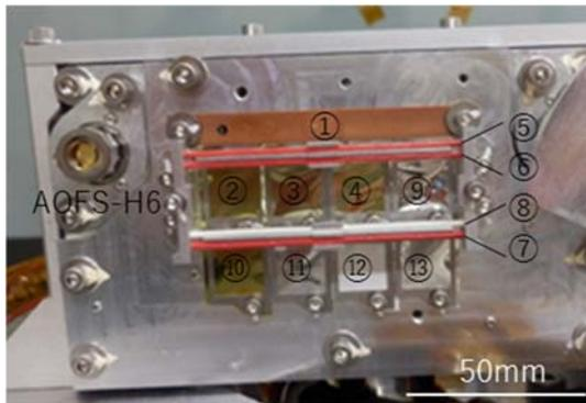
**Fig. 7.** Enlarged view of the MDM-S sample holding part and numbered mounting positions of material samples
