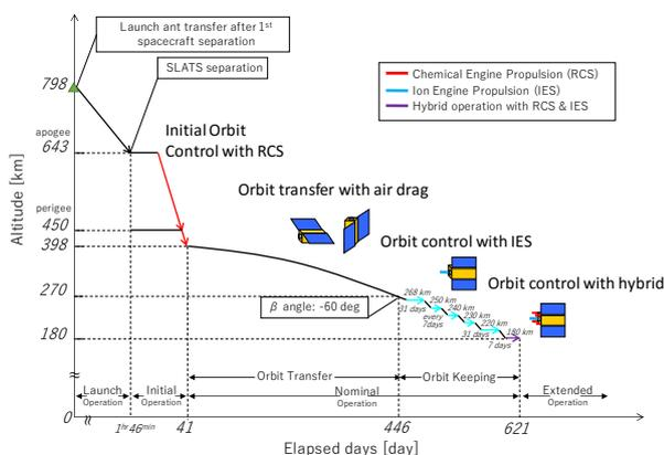
Fig. 2. Orbit transition profile plan of SLATS
