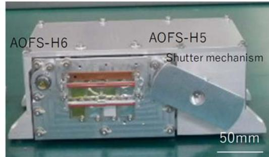
**Fig. 4.** MDM-S and AOFS-H (5 & 6; components also with a shutter mechanism)
