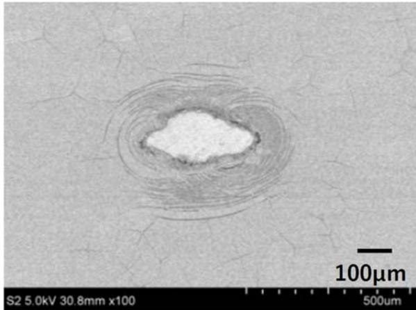
**Fig. 8.** SEM image of an impact hole due to MMOD on sample V
