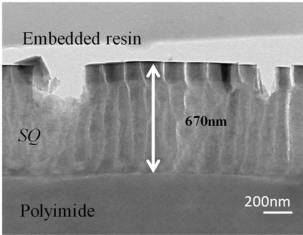
**Fig. 11.** TEM image of surface structure around an impact hole on sample V. Chippings or running cracks that occur vertically are those that occurred during the sample processing for TEM. Thus, these are artefacts not attributed to degradation by the space environment.
