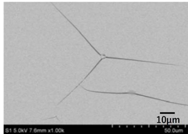
**Fig. 6.** SEM image of enlarged cracked portion on sample V
