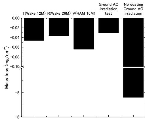
**Fig. 2.** Mass loss of the flight *SQ*-coated polyimide
