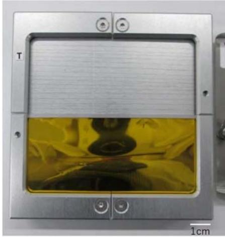
(a) One of the CNT flight configurations on ExHAM
