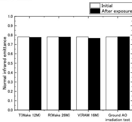
**Fig. 4.** Change in normal infrared emittance of the *SQ*-coated polyimide films
