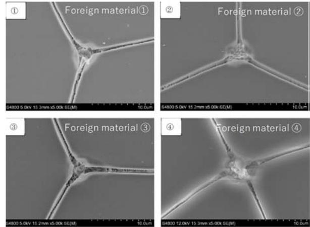
**Fig. 10.** SEM images of foreign materials in cracks on sample V
