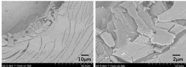
**Fig. 9.** SEM images of surface structures around an impact hole on sample V
