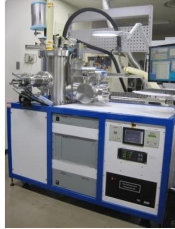
Fig. 2. Photo of outgassing rate measurement apparatus.
