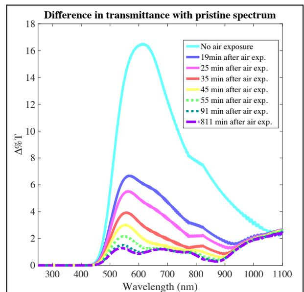
Fig 5 Difference in transmittance with the pristine sample spectrum before and after air exposure. Data were smoothed.
