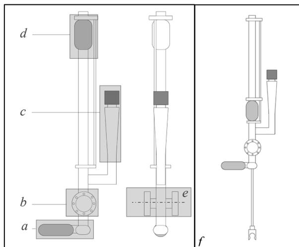
**Fig. 1** Diagram of the VTV showing: a) the gate valve b) optical window c) getter unit/ion pump d) magnetic feedthrough with rotation guide e) is the path of the measuring beam in the spectrophotometer f) the system with extended feedthrough arm and sample holder fork.
