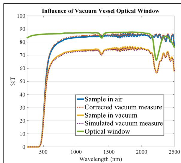
**Fig 2** Spectra of transmittance for optical window with and without sample in a vacuum and the calculated corrections. The correction of the spectrum in a vacuum fits the spectrum of the sample alone showing that the correction allows us to determine the spectrum of the pristine sample without interference from the optical window. Data were smoothed 50 times using the MATLAB smooth function.
