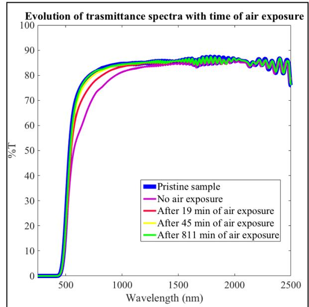
Fig 4 Evolution of transmittance after air exposure. Data were smoothed.
